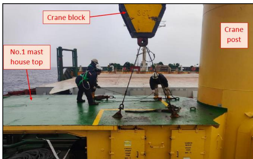
Figure 2 – Reenactment of securing No. 2 crane block to No. 1 crane platform after the occurrence ( Source: the Company, annotation by TSIB )
