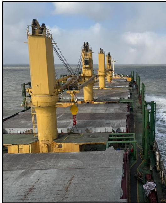
Figure 5 – View of the four cranes and their securing arrangements for sea passage looking forward ( Source: the Company )
