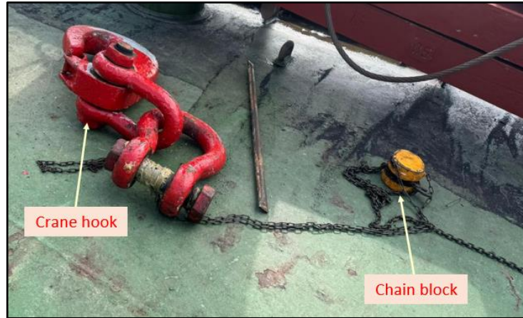
Figure 3 – The fallen No. 2 swivel hook with two D-shackles and chain block (Source: the Company, annotation by TSIB)
